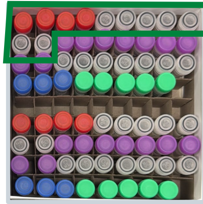
81-cell cryobox with 0.5 mL and 2.0 mL cryovials
