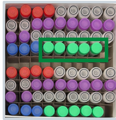
81-cell cryobox with 0.5 mL and 2.0 mL cryovials
